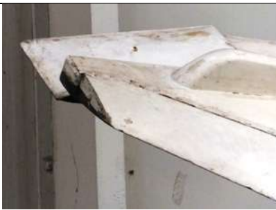
V2 rudder in tail fin and V2 graphite vanes in motor exit (RAF Museum Cosford)
