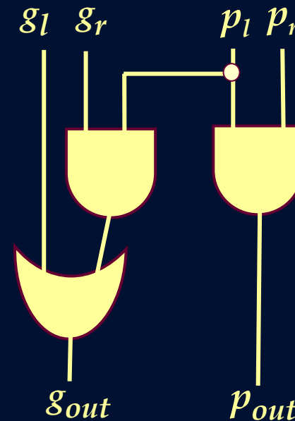
Gate-level implementation of P/G block
