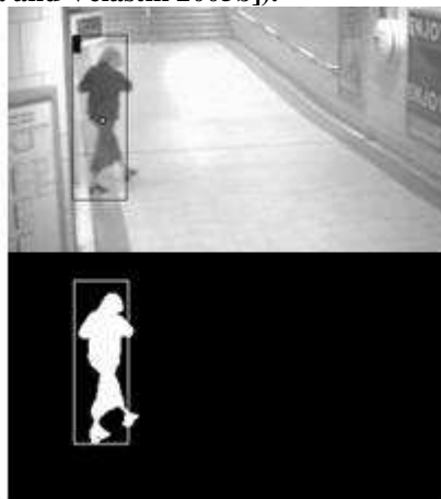
Figure 2- 3. Example of a background subtraction technique used in motion detection. In this example a bounding box is drawn to fit the object detected (from [Valera and Velastin 2005b]).
