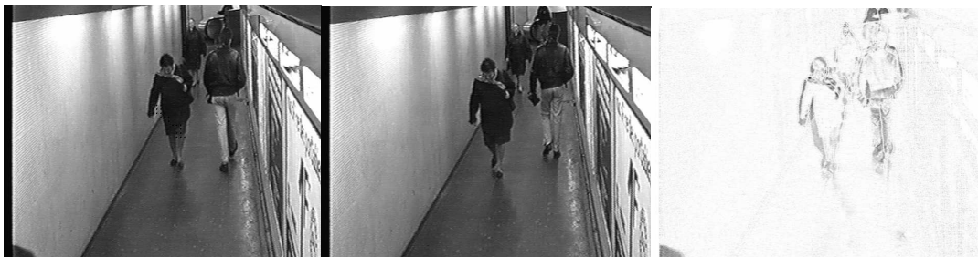
Figure 2- 2. Example of a temporal difference technique used in motion detection (from [Valera and Velastin 2005b]).
