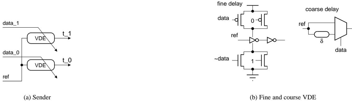
Figure 5: Block diagram of the sender and implementation examples of VDE
