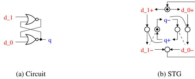
Figure 5.14: Single-spacer dual-rail to single-rail converter
