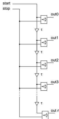
Figure 1: Delay line-based TDC
