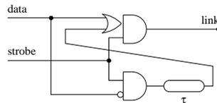
Figure 4: Block diagram of PWM sender
