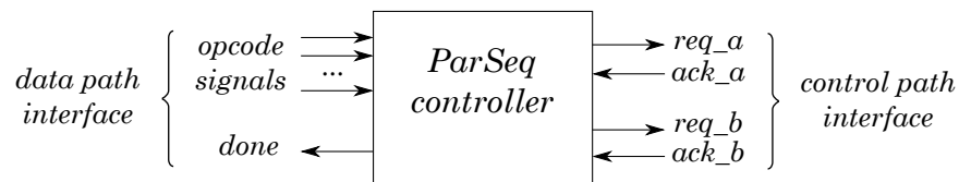
Figure 3.1: ParSeq controller interface
