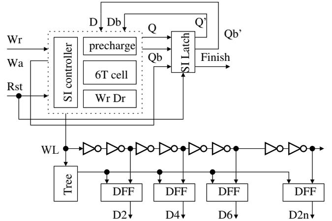
FIGURE 10 BLOCK DIAGRAM OF THE PROPOSED SENSOR.
