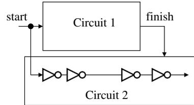
FIGURE 6 THE REFERENCE FREE SENSOR MECHANISM.
