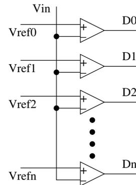
FIGURE 3 BLOCK DIAGRAM OF FLASH ADC.
