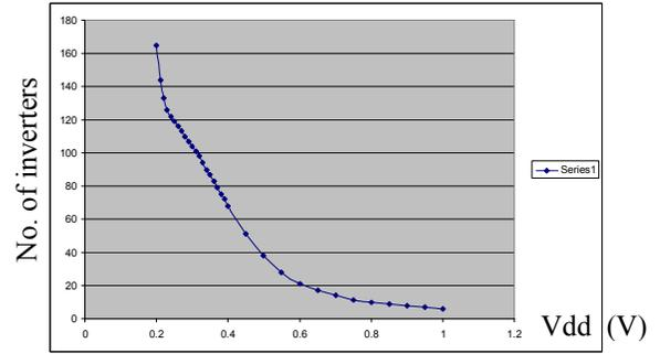
FIGURE 12 MEASUREMENT RESULTS FOR MODIFIED THRESHOLD INVERTERS.
