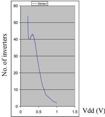
FIGURE 11 VDD VS. INVERTER COUNT.
