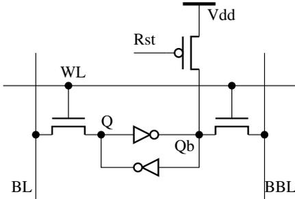
FIGURE 9 MODIFIED 6T SRAM CELL.
