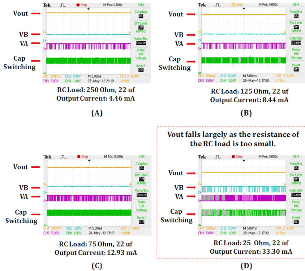
Figure 27. 1.2 V regulated power delivered to an adjustable RC load.
