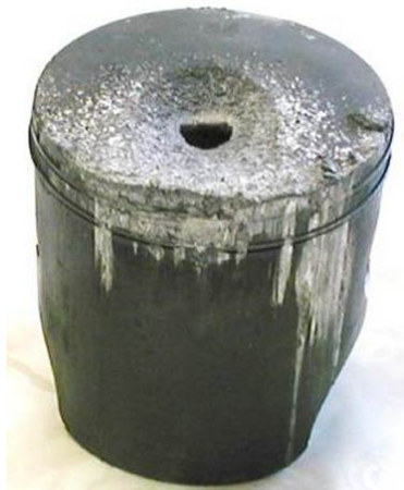
Figure 5.3: Piston Damage caused by late ignition
