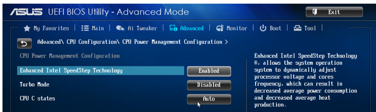
Figure 9: BIOS screenshot showing SpeedStep enabled and C states in auto mode
